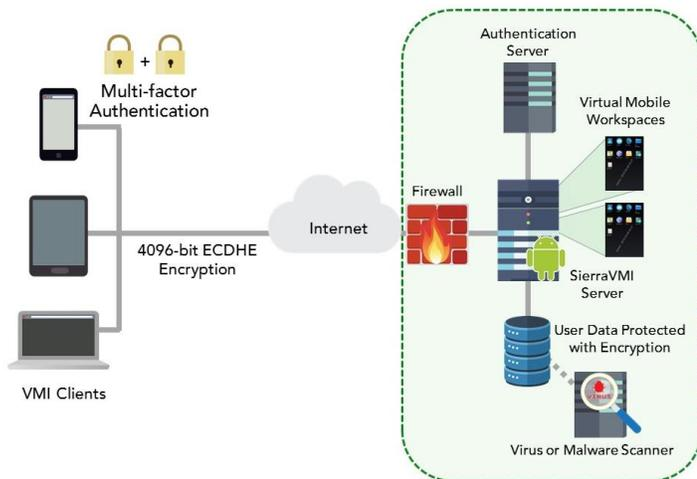
*A VMI deployment, with phones, tablets and laptops accessing a VMI server hosting mobile apps remotely.*
